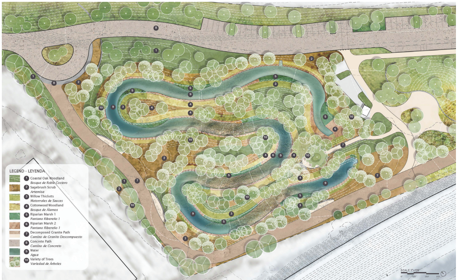
FIGURE 19. Bowtie Demonstration Wetlands conceptual design, which includes a diverse range of habitats and species, a looping channel for water to pass through, and walkways along the constructed wetlands.
