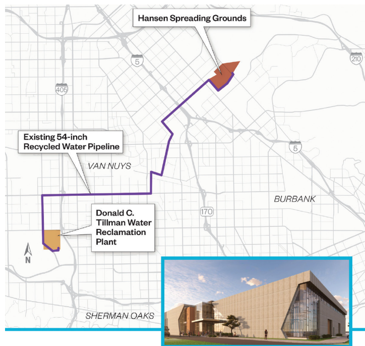
FIGURE 18. Map of infrastructure leading recycled water from Donald C. Tillman Water Reclamation Plant to the Hansen Spreading Grounds.
